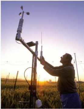
Feedback from wind sensors helped Bruce Kimball control the release of CO<sub>2</sub> in a FACE study on wheat.
